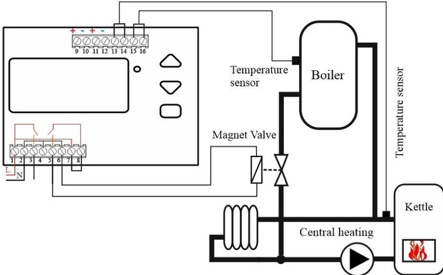
**D) Heating of the boiler by the fireplace and electric heaters**
